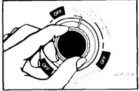
**B.** Stop on a number in the cycle you want. The numbers are minutes of wash time. The drawing shows 8 minutes of agitation in the REGULAR HEAVY Cycle. **NOTE:** In the REGULAR HEAVY and SHORT Cycles, the washer will fill only when the knob points to a "fill" area.
